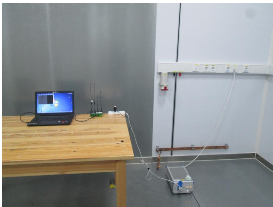
Fig. 4 Power line conducted emission setup photo
