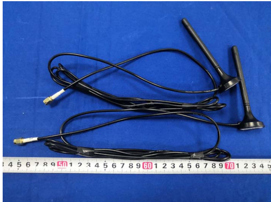
LTE Antenna View
