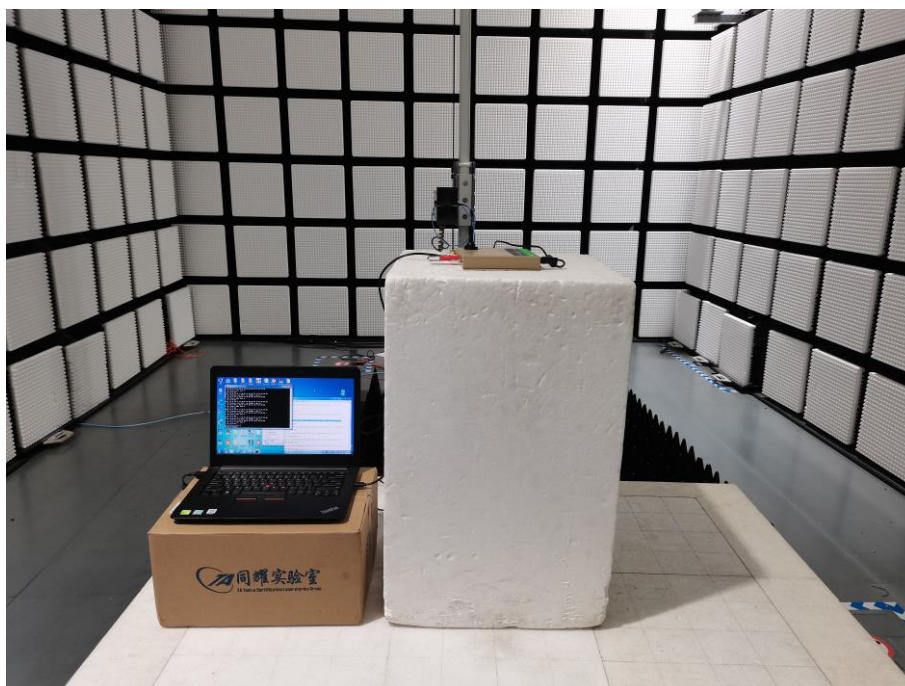
Fig. 3 Radiated emission setup photo(Above 1GHz)
