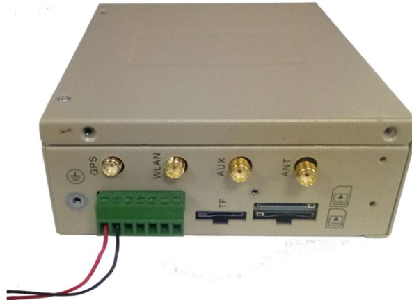
Figure 3-7 Installing the Power Supply
