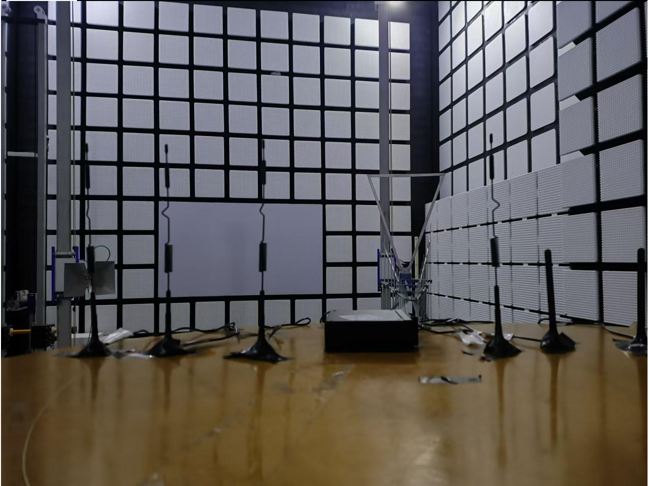
RF Radiated Test setup (RSE)
