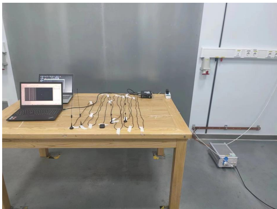
Power line conducted emission setup photo
