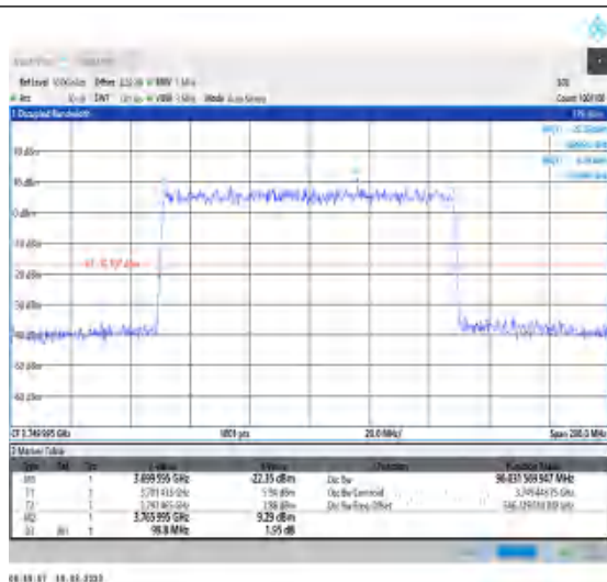
1-N78-3700-3800-30-100-L-5-DFT-256QAM- Outer Full-270@0-Ant0-96.032-99.800-≤100-PASS
