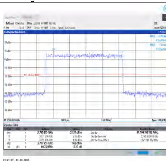
1-N78-3700-3800-30-70-H-5-DFT-256QAM- Outer Full-180@0-Ant0-64.2-66.220-≤70-PASS
