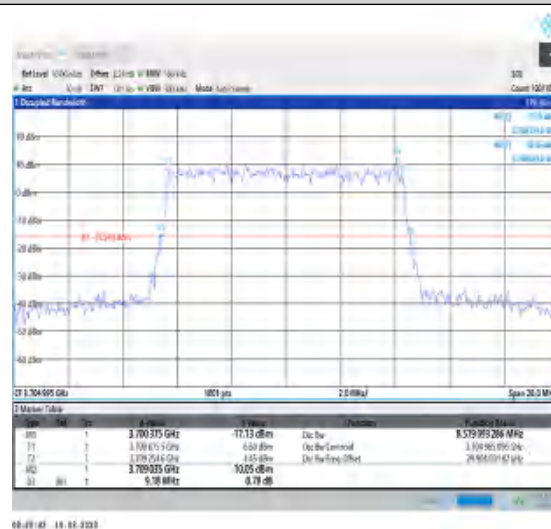
1-N78-3700-3800-30-10-L-4-DFT-64QAM- Outer Full-24@0-Ant0-8.579-9.180-≤10-PASS
