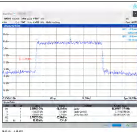
1-N78-3700-3800-30-90-L-4-DFT-64QAM- Outer Full-240@0-Ant0-85.594-88.920≤90-PASS
