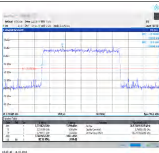
1-N78-3700-3800-30-80-H-5-DFT-256QAM- Outer Full-216@0-Ant0-76.976-80.160-≤80-PASS
