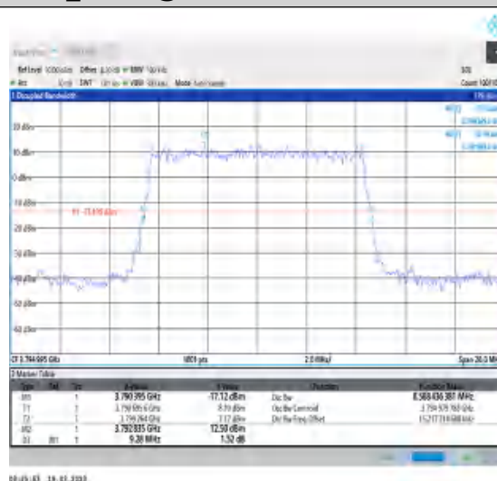
1-N78-3700-3800-30-10-H-2-DFT-PI2BPSK- Outer Full-24@0-Ant0-8.568-9.280-≤10-PASS
