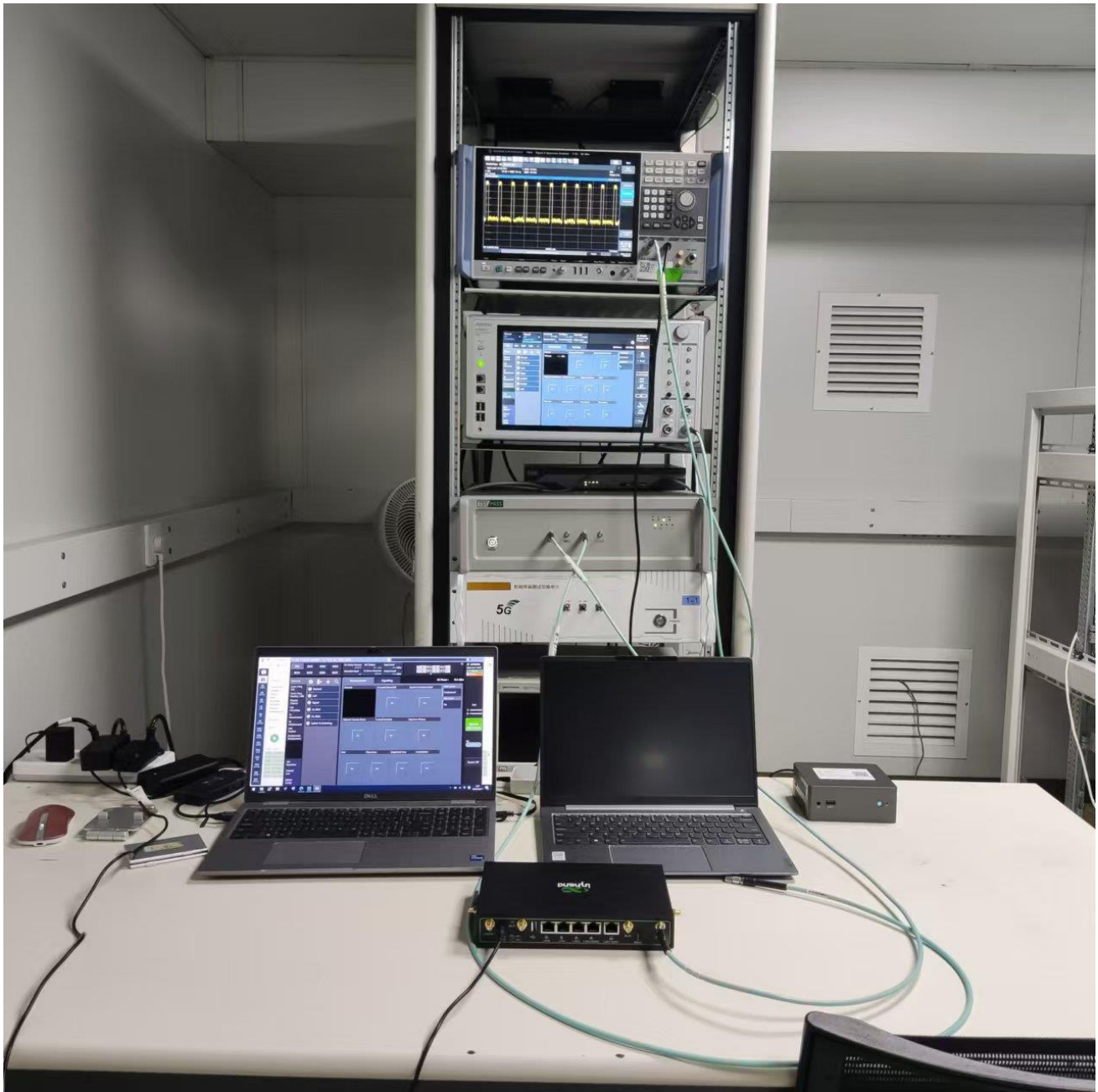
RF Conducted Test setup (LTE/NR)
