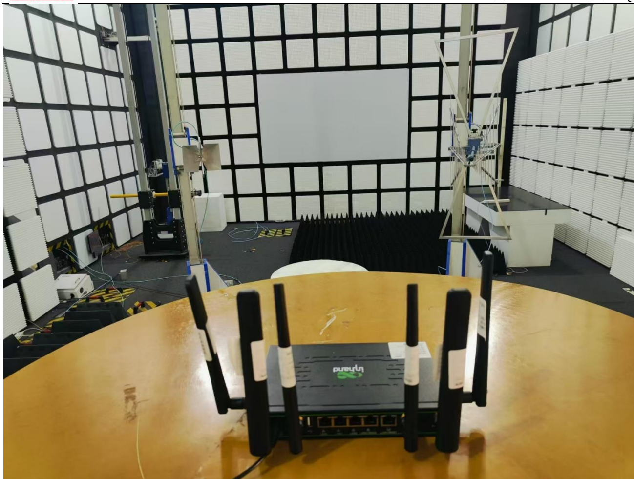
RF Radiated Test setup (RSE)
