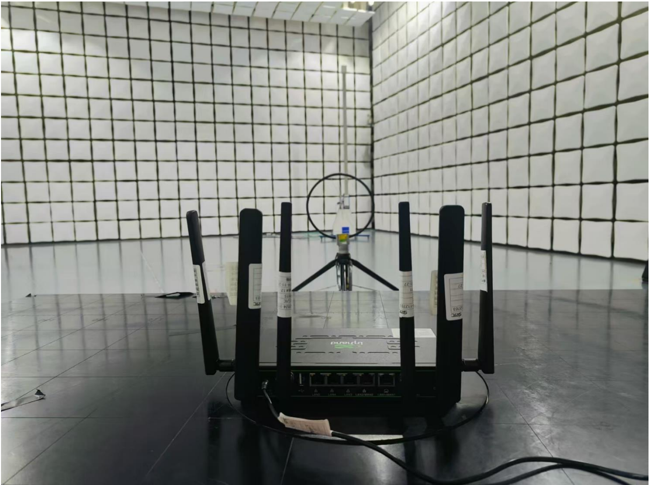
RF Radiated Test setup (9KHz~30MHz)
