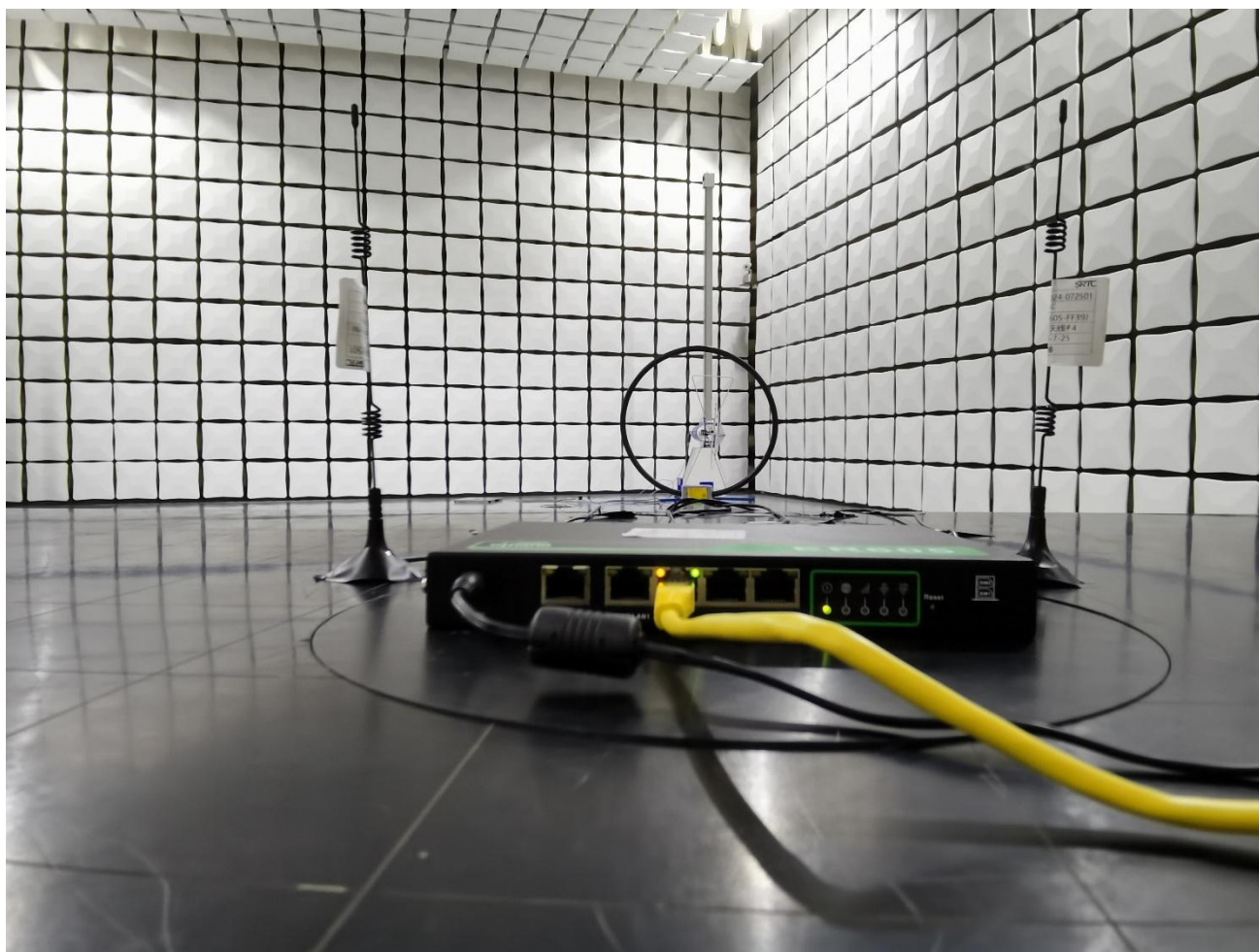
RF Radiated Test setup (9KHz~30MHz)
