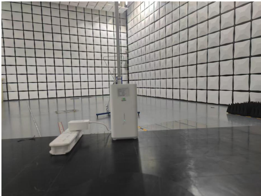
Radiated Emissions Test Setup (with charger) (30-1000MHz)
