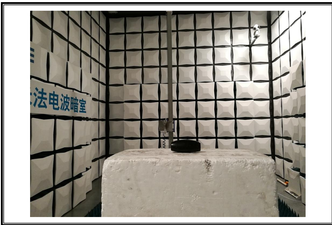
RADIATED RF MEASUREMENT SETUP (ABOVE 1 GHz)
