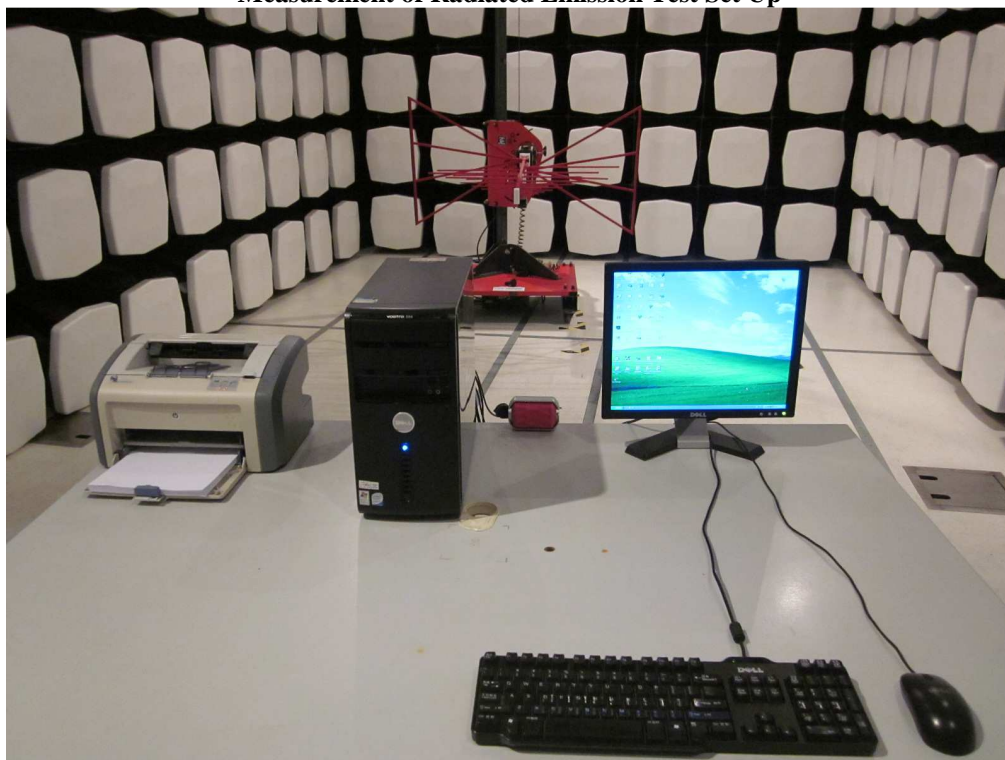
Measurement of Radiated Emission Test Set Up
