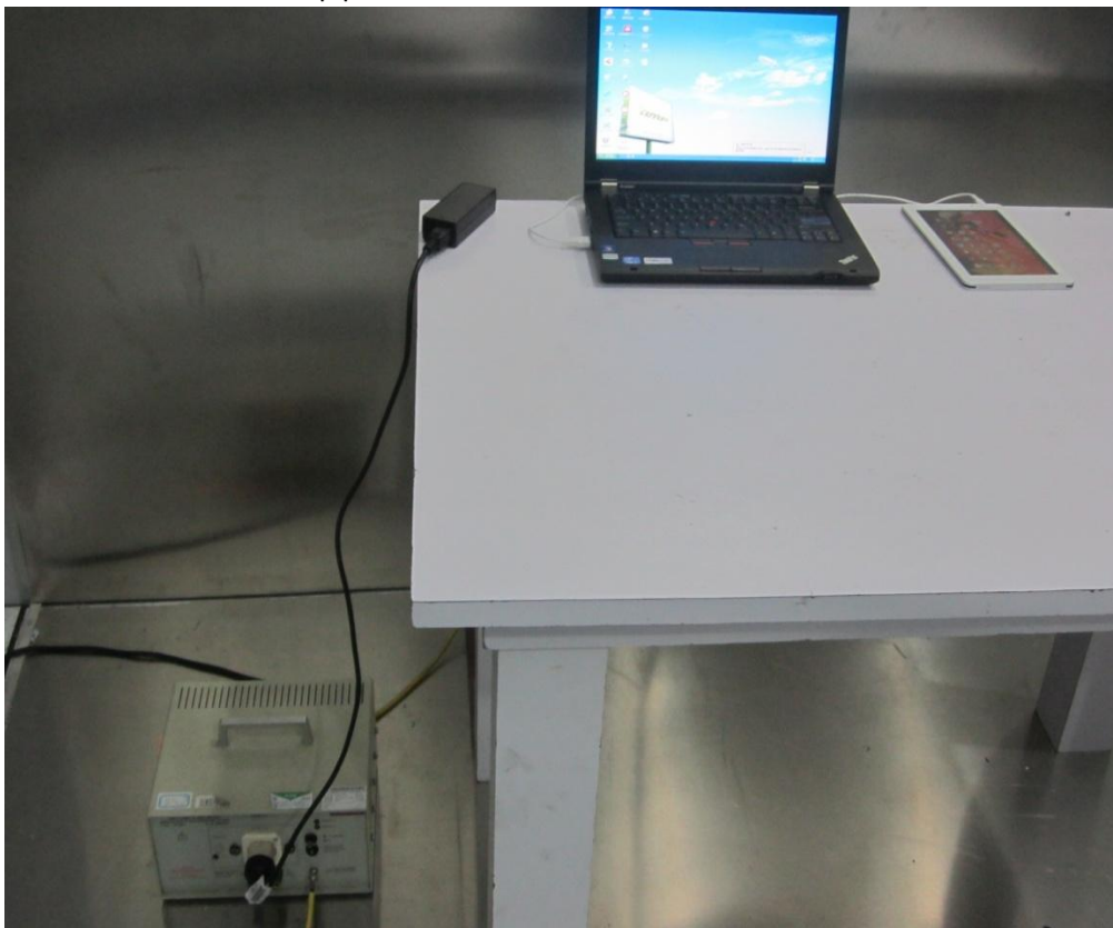
Conducted Emission Test setup photo
