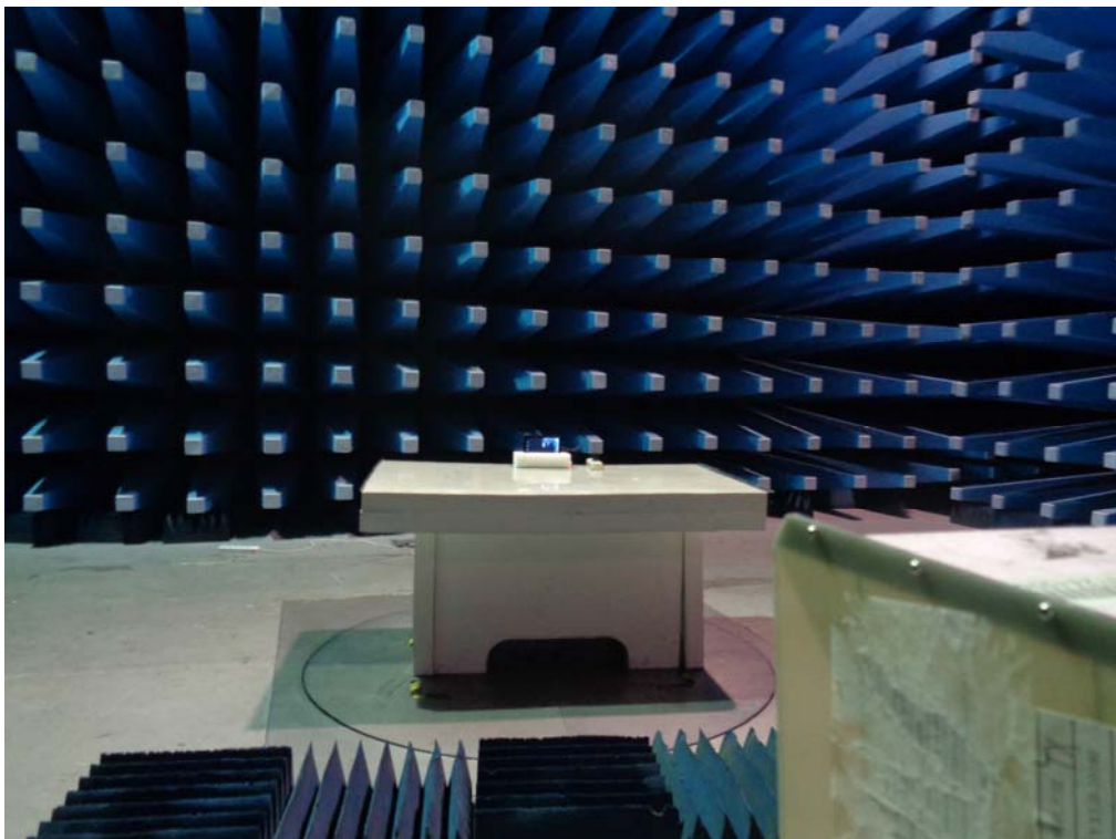
Radiated Spurious Emissions Test Setup Below 1GHz
