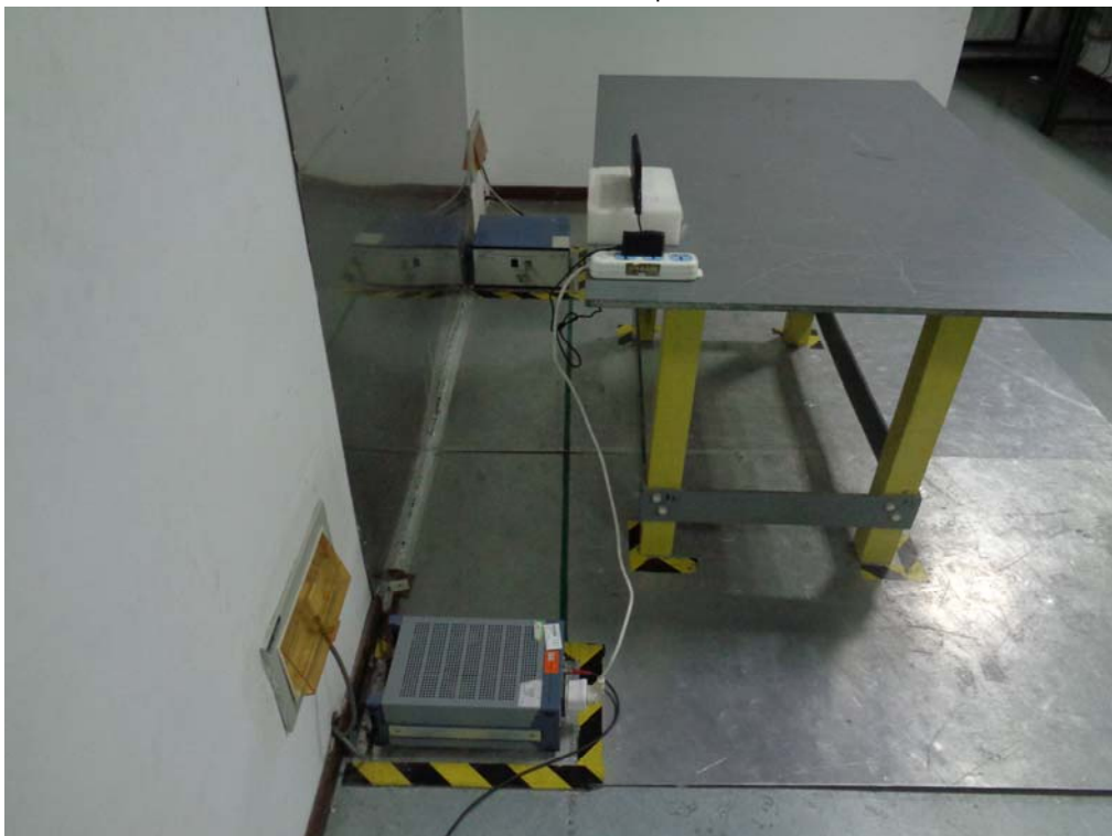
Conducted Emissions Test Setup – Side View
