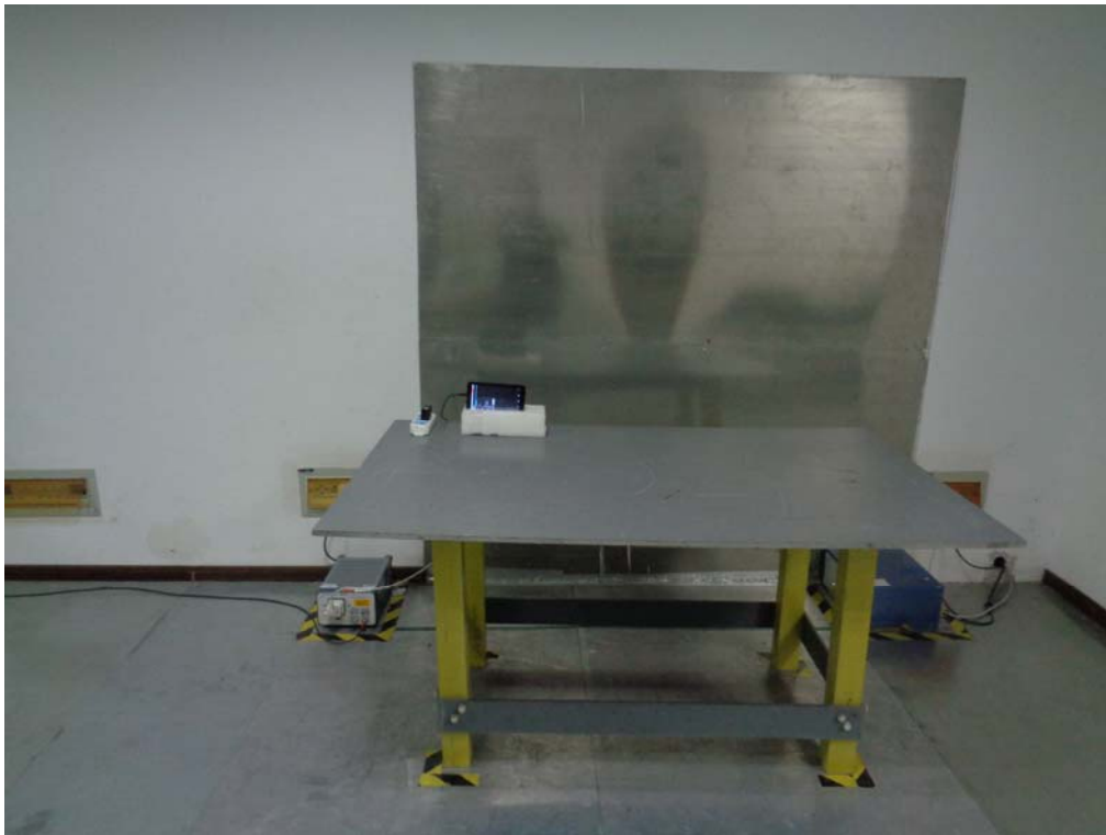
Conducted Emissions Test Setup – Front View
