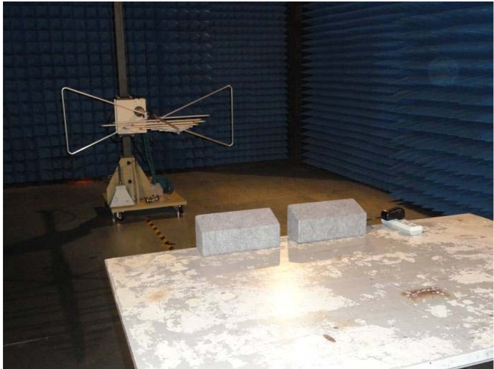
Radiated Emission Test Setup:
