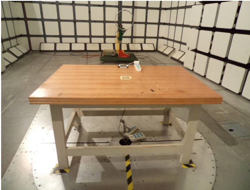
Radiated Emissions – Front View (Below 30 MHz)
