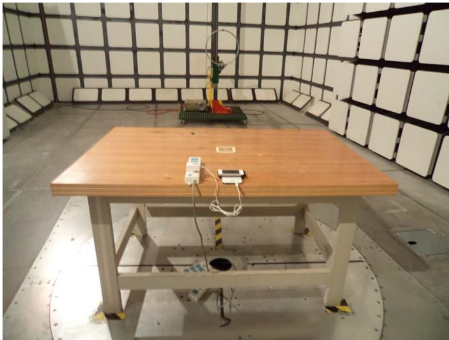
Radiated Emissions – Rear View (Below 30 MHz)
