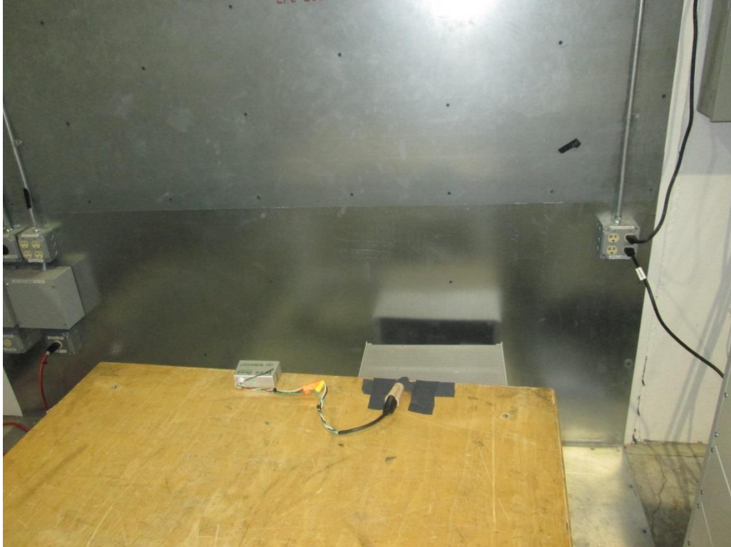
Conducted Emissions, AC Mains, Front View
