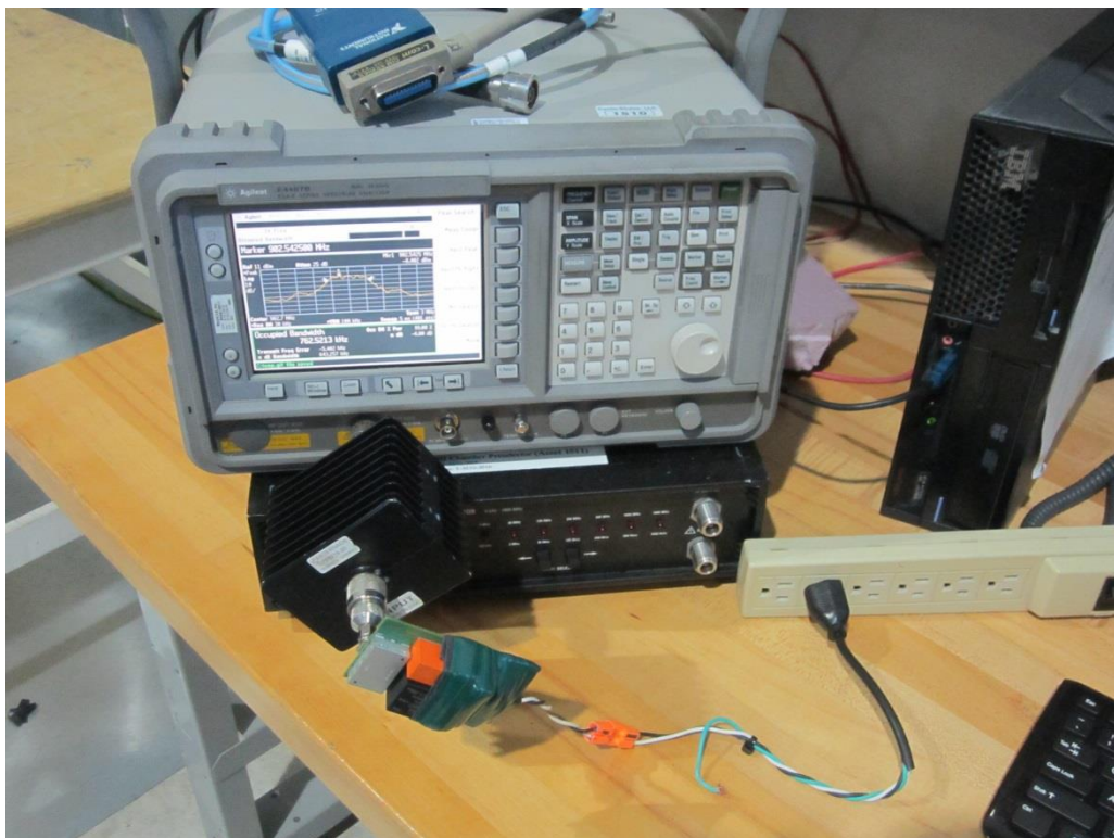
Band Edge, OBW, 6dB BW, PSD, POP Test Setup
