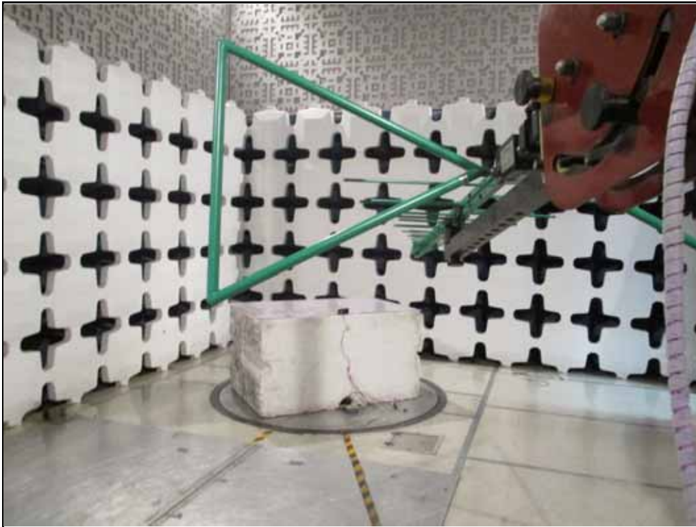
Test Setup for Effective Isotropic Radiated Power – Horizontal Polarization
