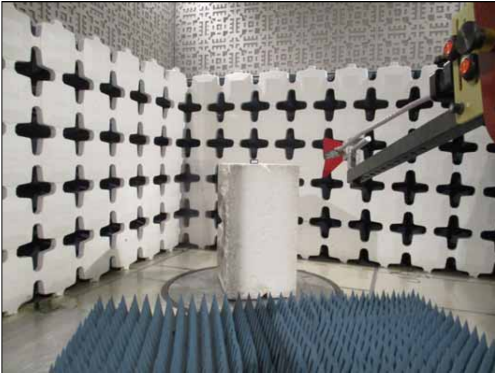
Test Setup for Spurious Radiated Emissions above 1GHz – Horizontal Polarization
