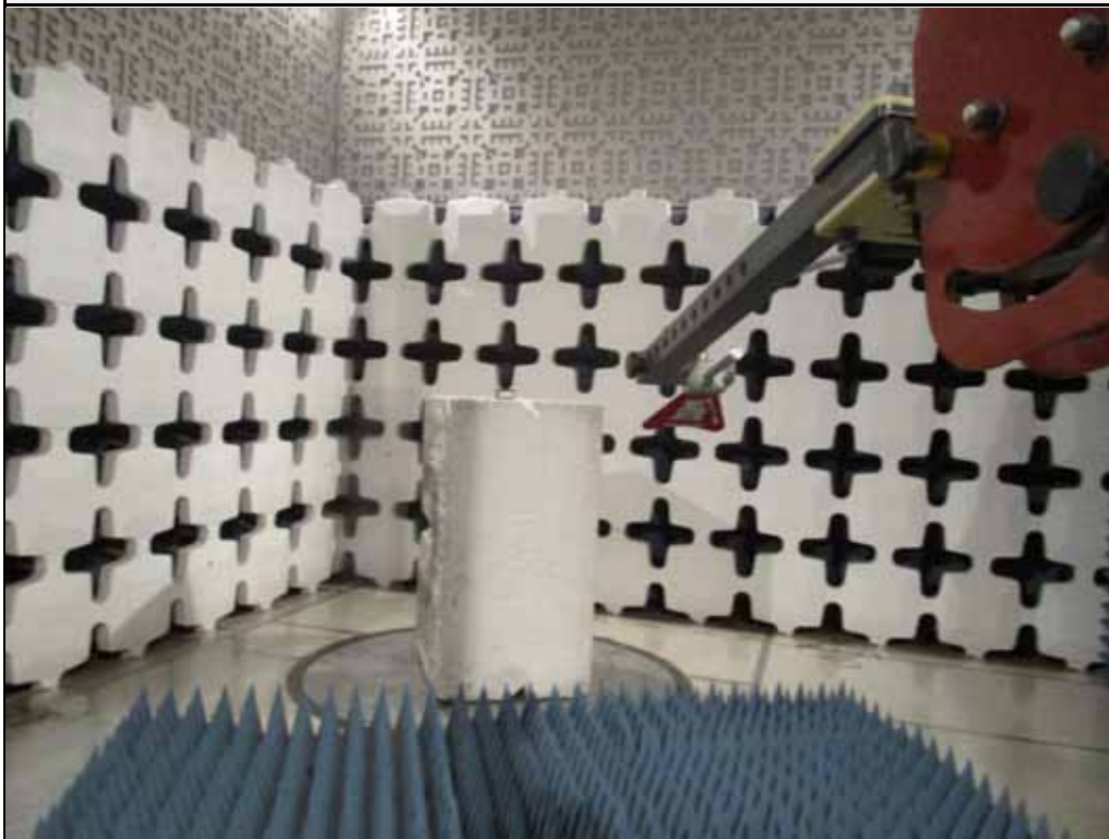
Test Setup for Spurious Radiated Emissions above 1GHz – Vertical Polarization
