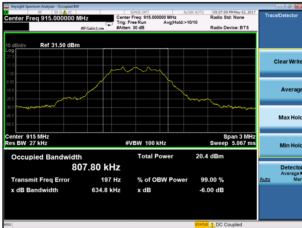
Occupied Bandwidth – Middle Channel
