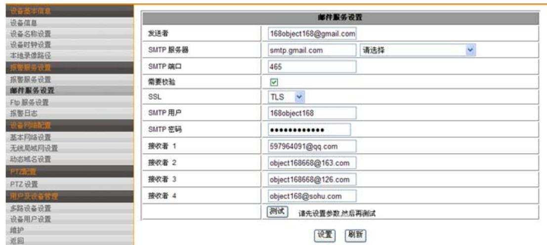
This function is to alarm by send emails. If the camera alarms, it will automatically send emails to the email address preset.
