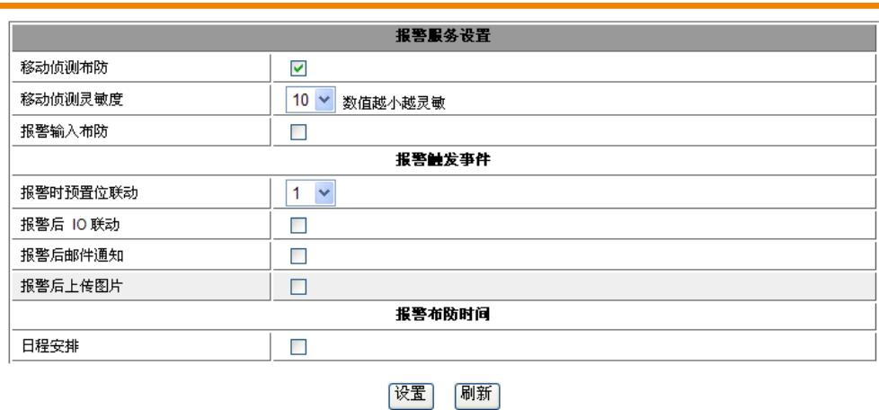
Choose the way for alarm, whether it's IO linkage, send email, upload image, or linkage presetting position alarm. Example: motion detection all day monitor, set the
