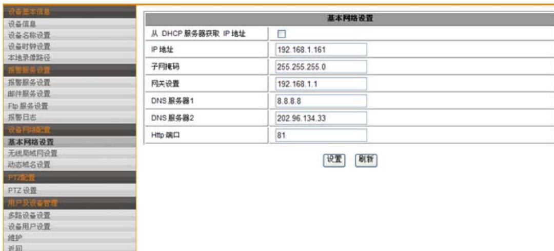
Set the sub network mask, gateway, DNS server before use. When like below choose DHCP, device will get the IP address automatically.
