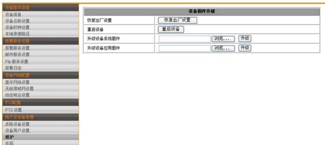
Click **恢复出厂设置**, the device would restart and renew to the defaulted setting from factory
