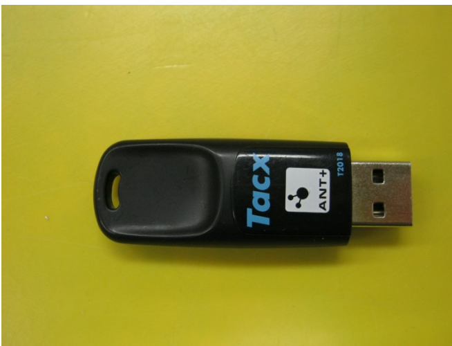
Photograph 2.3-3: Top view of ANT+ USB Stick used for test mode running
