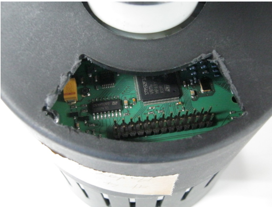
Photograph A2-8: Detail view Sample #4, housing opened for connection to terminal
