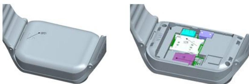
Please refer to above drawings for how to install a SIM card and Micro SD card.
