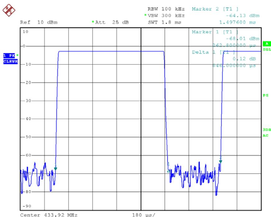
**Note:** “Marker 1” means the moment button was persistent pressed, and “Marker 2” means where the transmitter deactivated automatically.
