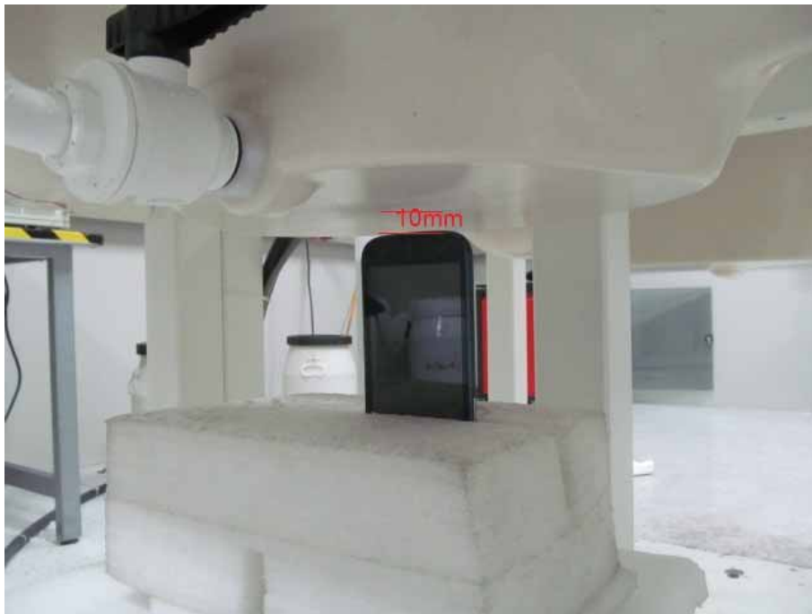
Body SAR Bottom 10mm for GSM/UMTS
