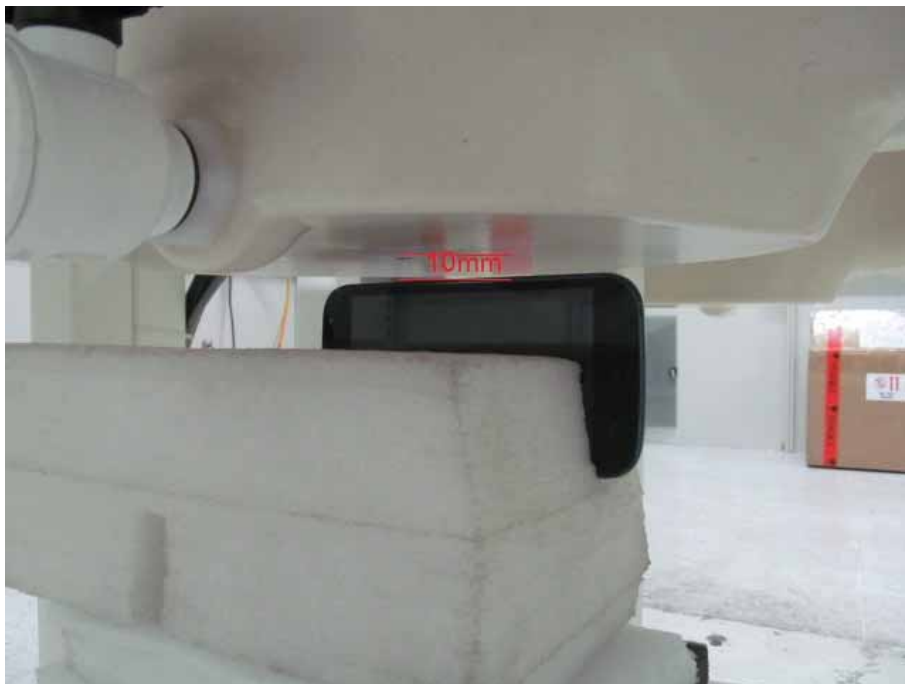
Body SAR Right Side 10mm for GSM/UMTS
