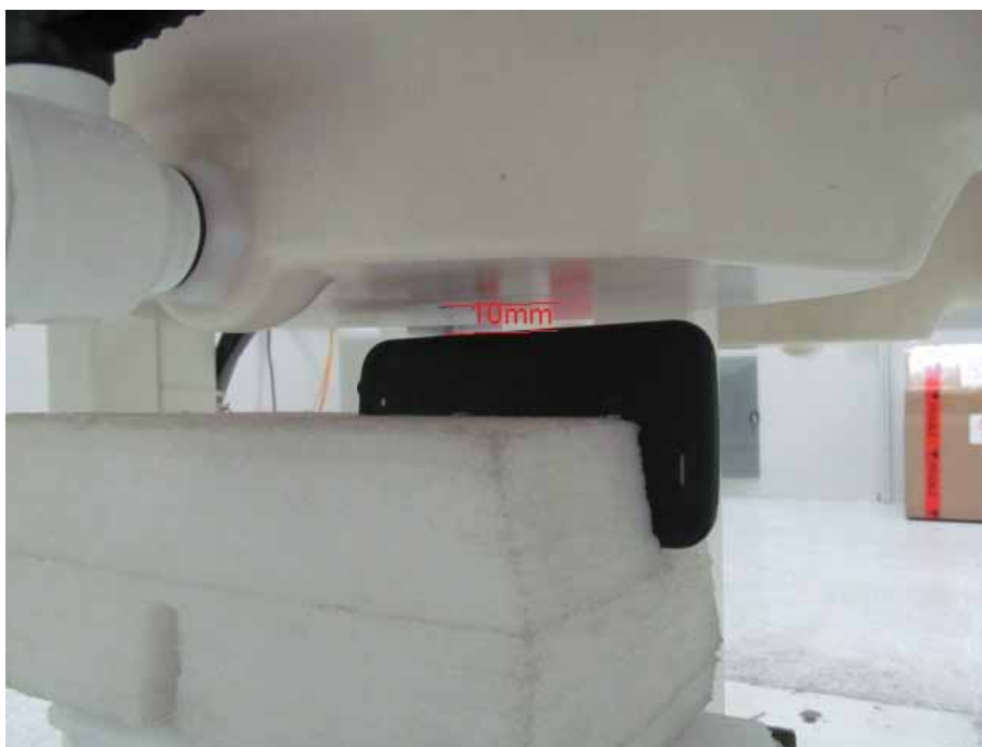
Body SAR Left Side 10mm for GSM/UMTS
