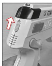
The G8 Pro V2 is a sophisticated piece of electronic equipment. Similar to a mobile phone, it has a boot-up cycle. This boot-up cycle lasts approximately 30 seconds. The Battery Capacity Gauge's green LEDs temporarily illuminate once G8 Pro V2 has completed its boot-up cycle and is ready for use. (After the unit has been successfully paired with a mobile phone, it will "beep" twice to indicate the boot-up cycle is complete and the unit is ready for use.)
