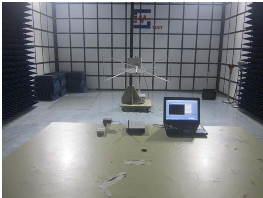
**Radiation Emission Test Setup (Above 1GHz)**
