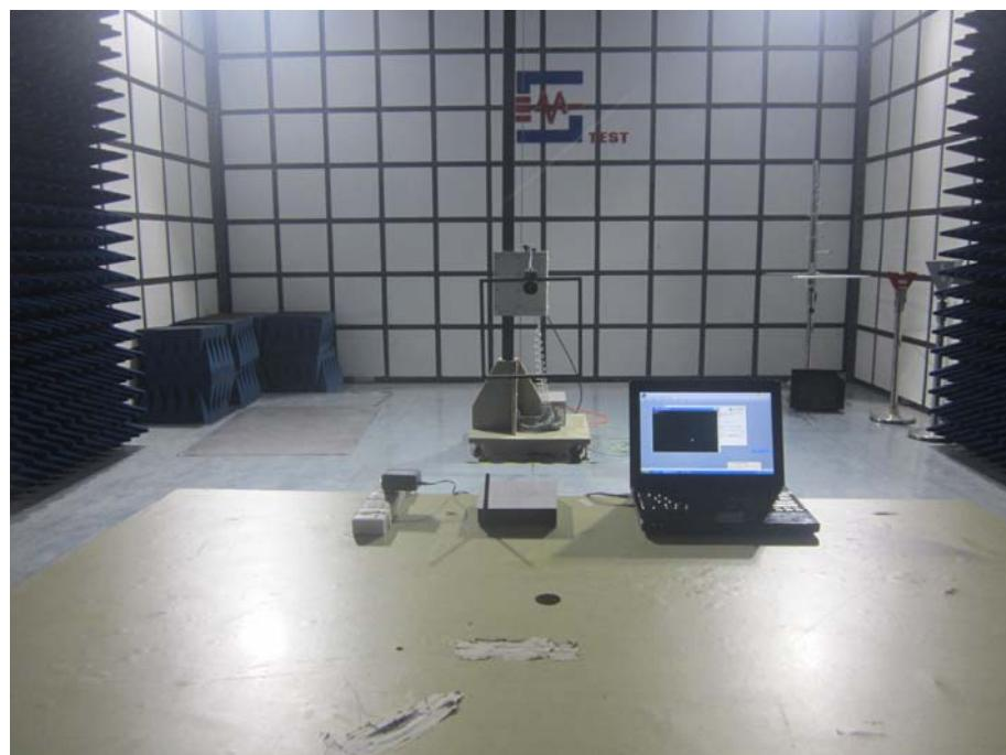
**Radiation Emission Test Setup (30MHz to 1GHz)**
