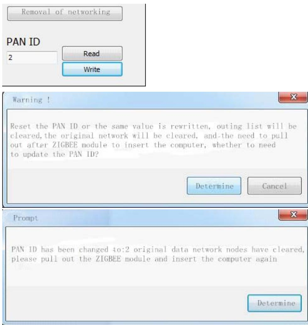
Point after "ok", pull out the Zigbee module, and then reinsert the computer.
