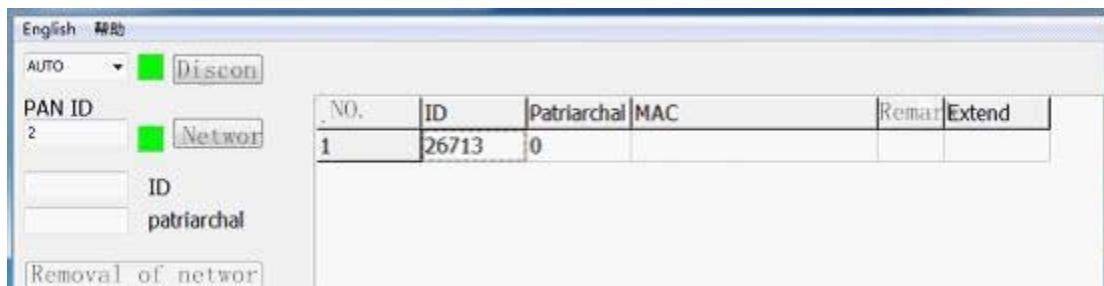
6、After the success of the network, double-click the window under the "26713" the projector to do "normal, KeySton, LenzShift, fusion splicing" operation, the following figure:
