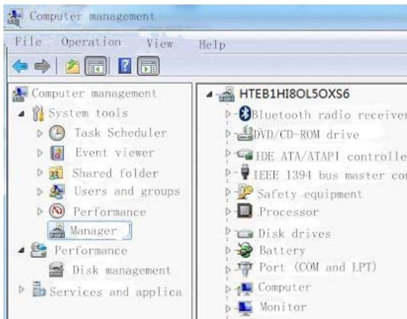
After opening the "port (COM and LPT)" item, see "Silicon Labs CP210x USB to UART Bridge (COM7)" Words, COM7 is our the port to be used.
