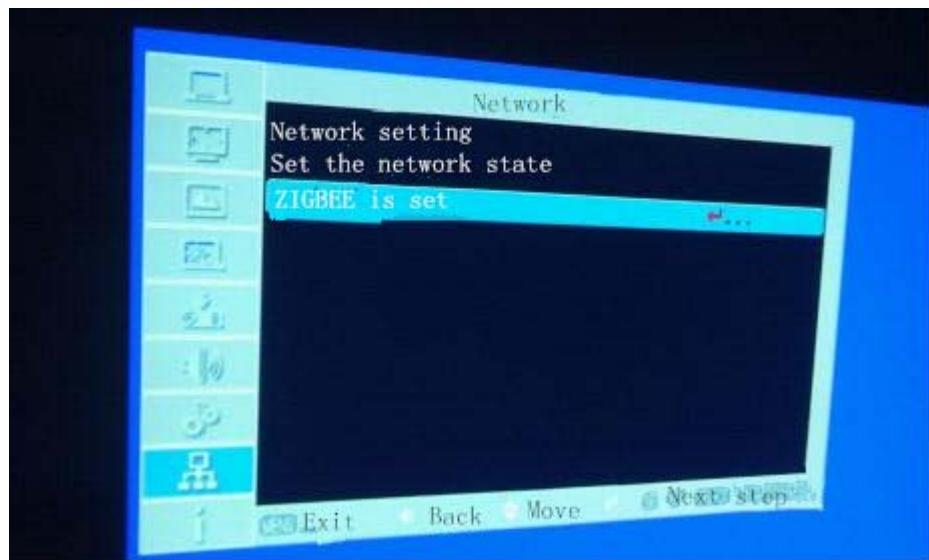
Sets the "Zigbee mode" to "open", press "OK" button on the remote control; Will be set to "PAN ID" and the computer terminal window under the same "2" and press "OK" button on the remote control, the following figure:
