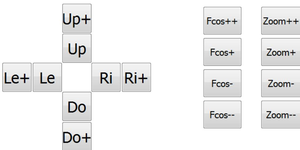
When entering "Lenzshift", whenever shift in one direction, should be first "coarse" button operation, such as: the Up +, Do +, Le +, Ri +, then adjust "fine tuning" buttons, such as: Up, Do, Le, Ri.
