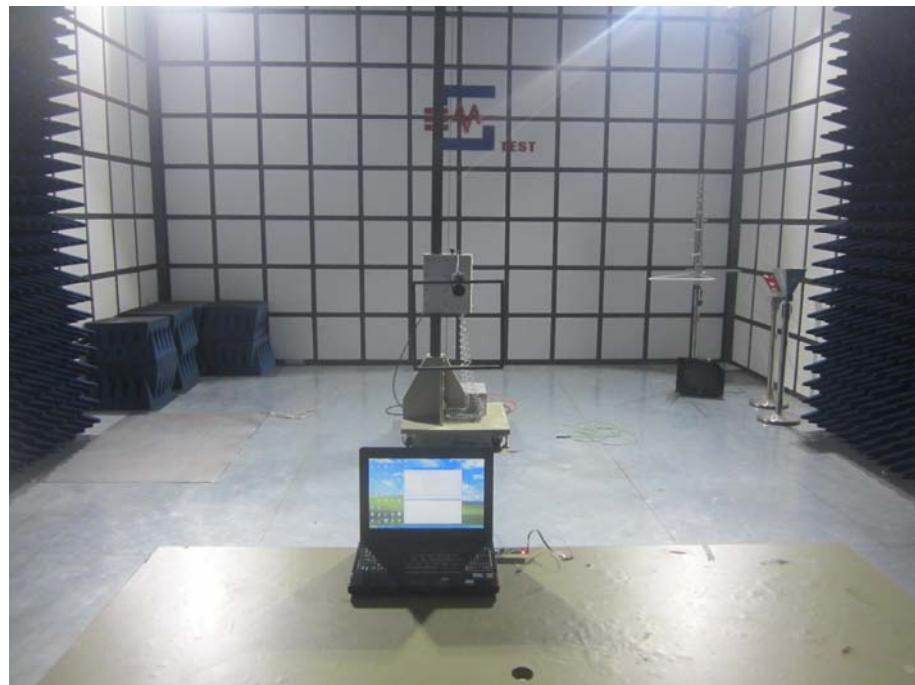
**Radiation Emission Test Setup (Above 1GHz)**
