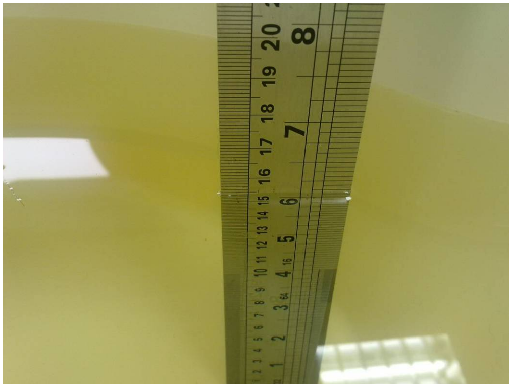
Liquid depth in the Flat Phantom (2450MHz)
