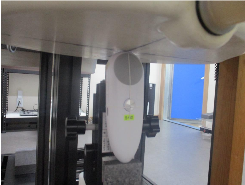
Top Side from Flat Phantom (Separation Distance: 0 cm) – Body SAR
