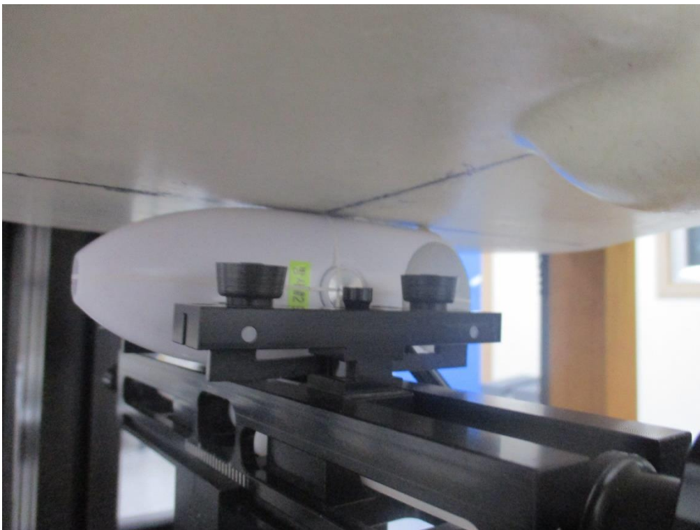
Left Side from Flat Phantom (Separation Distance: 0 cm) – Body SAR
