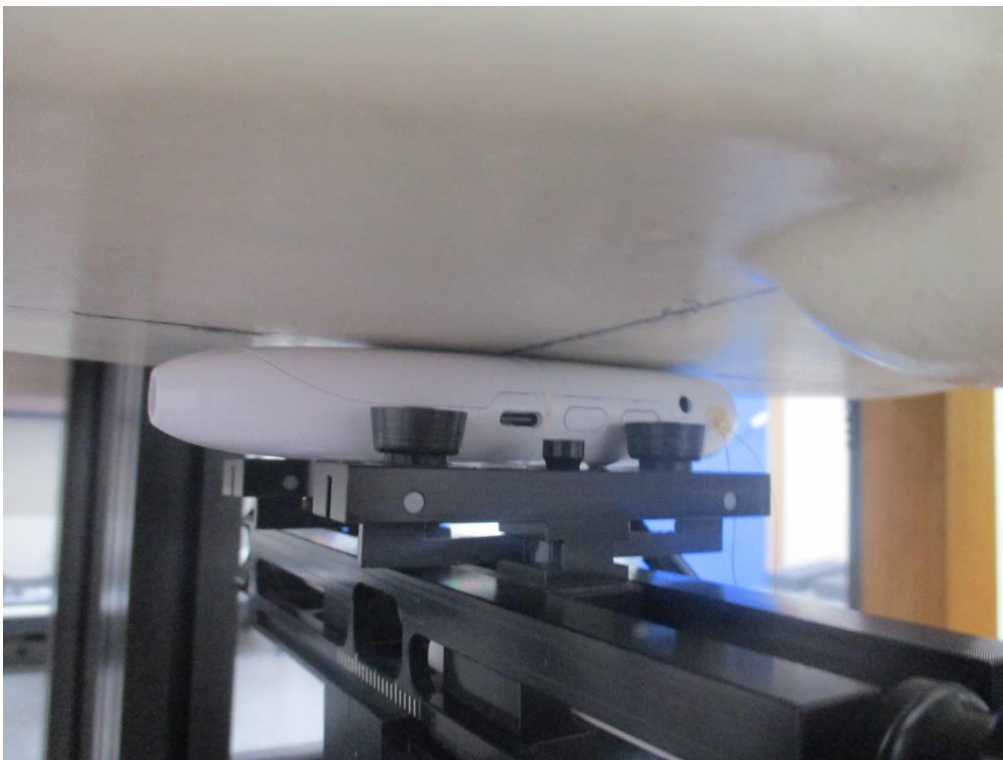
Rear Side from Flat Phantom (Separation Distance: 0 cm) – Body SAR
