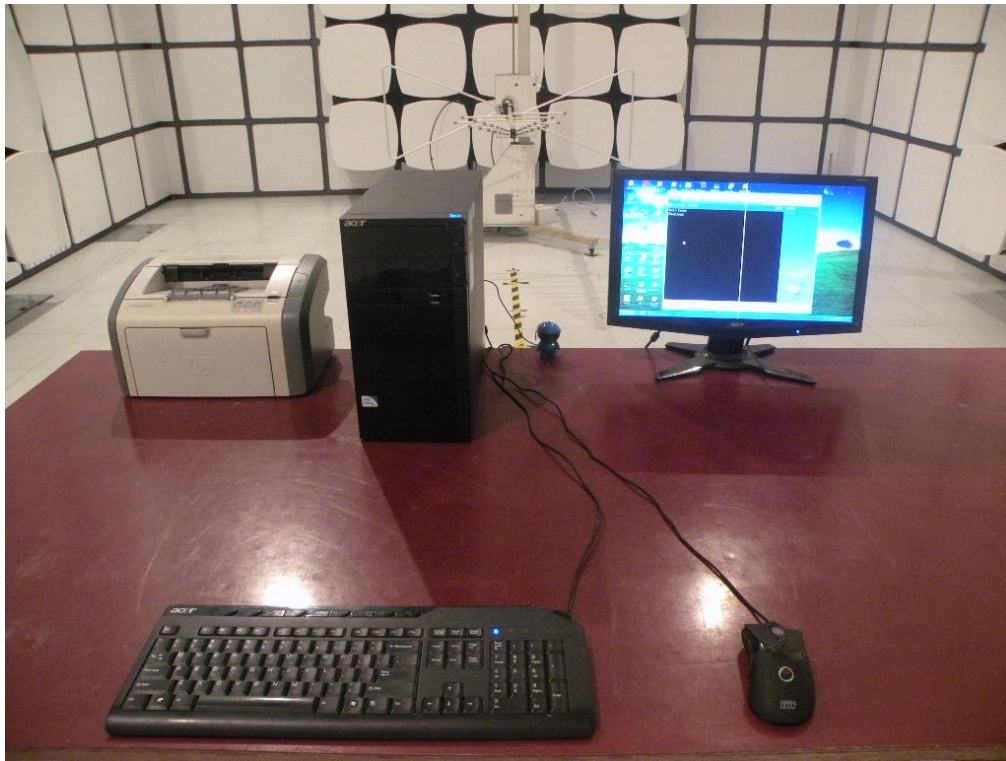
Radiated Emission Test Setup in Chamber
