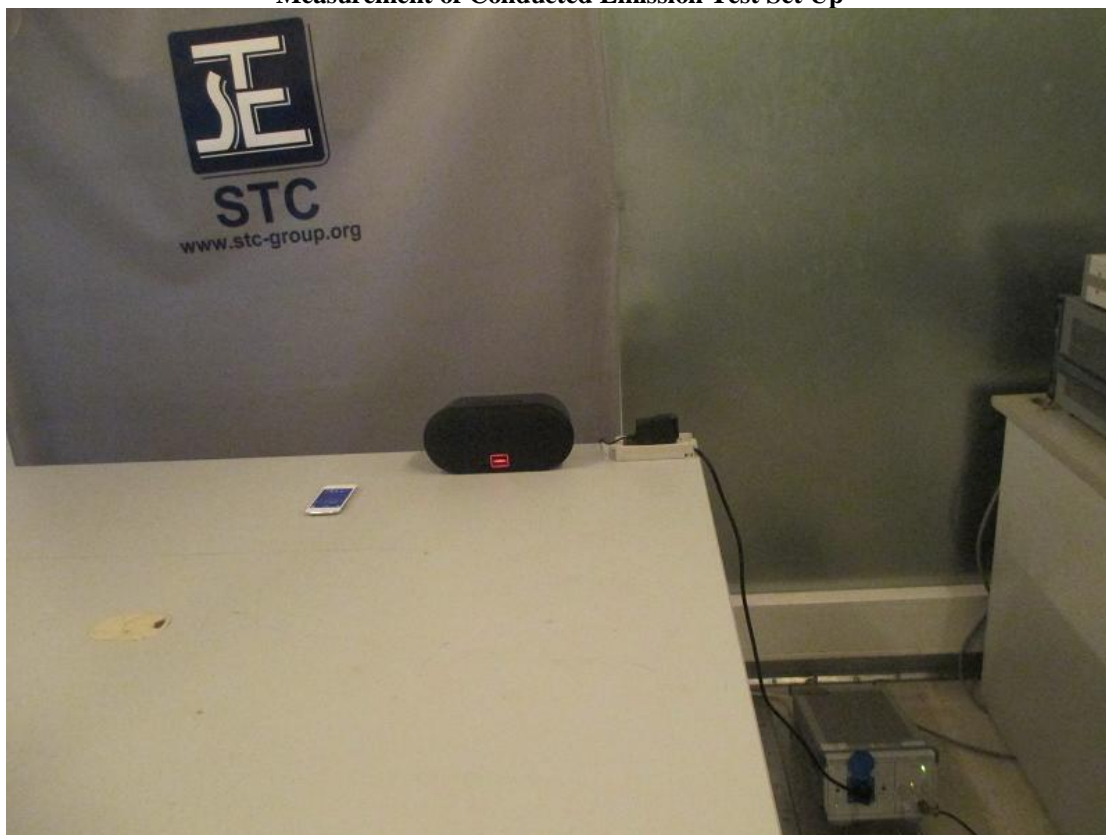
Measurement of Conducted Emission Test Set Up
