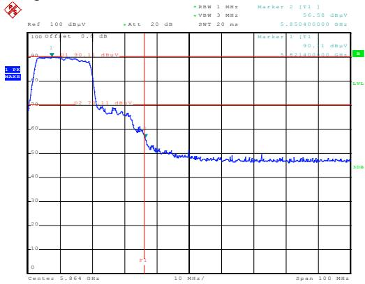
Figure 4. Plot of the Spurious RF conducted emissions
