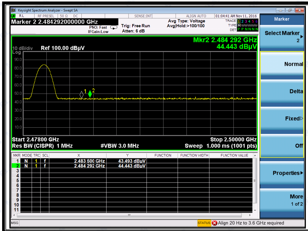
(Plot B1: Channel = 78 PEAK @ GFSK)
