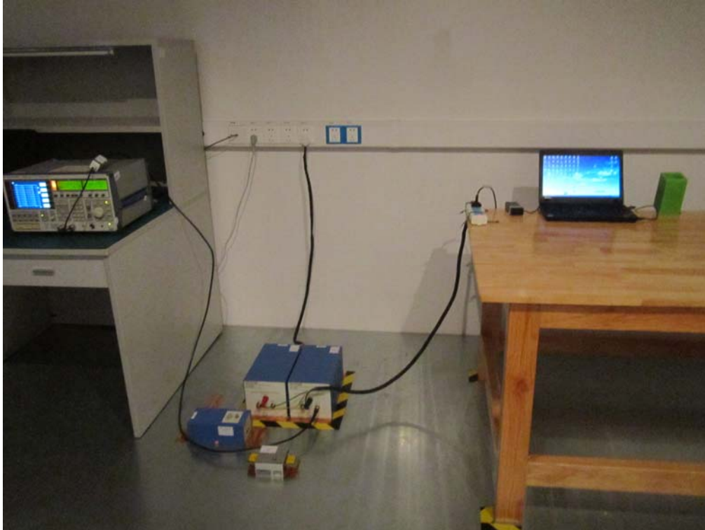
Conducted Emissions Test Setup Front View
