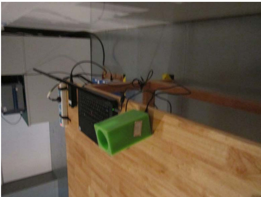
Conducted Emissions Test Setup Side View
