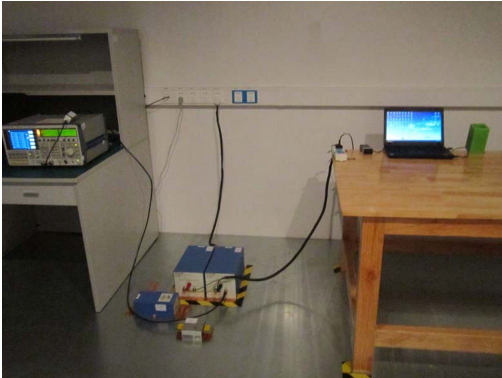
Conducted Emissions Test Setup Front View
