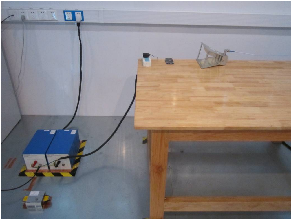
Conducted Emissions Test Setup Front View
