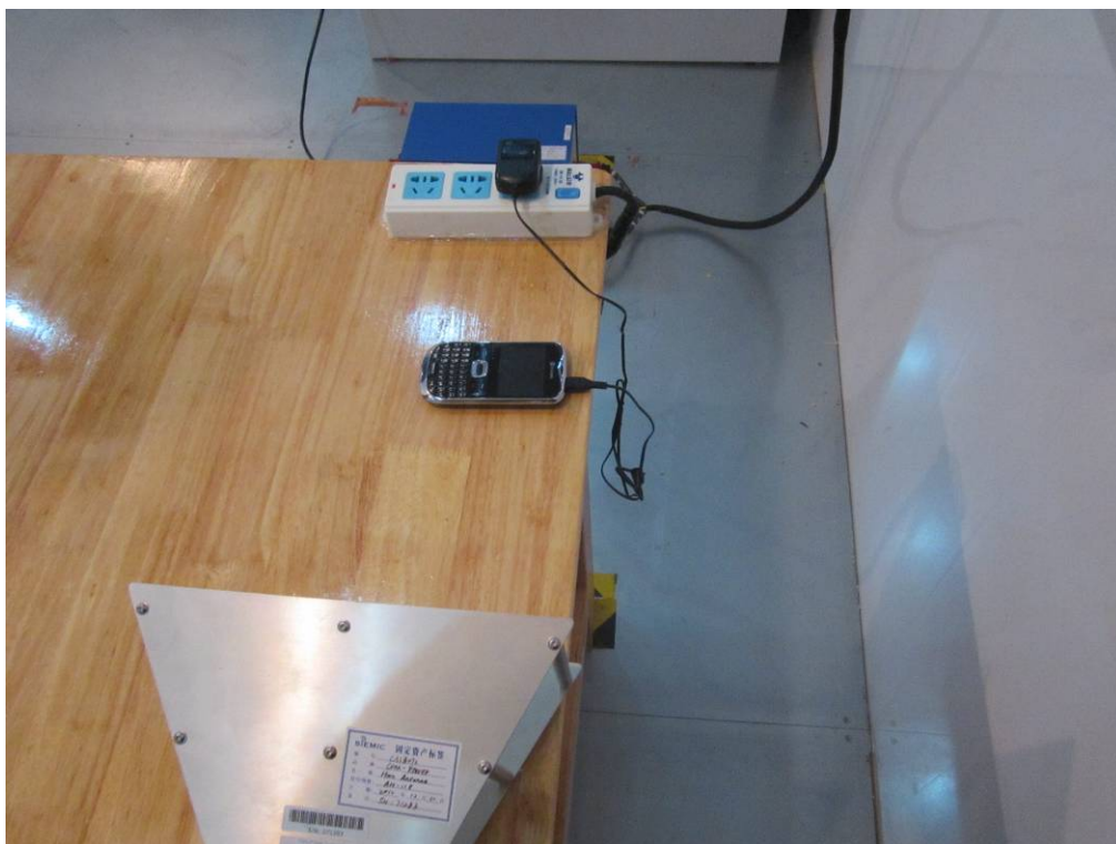
Conducted Emissions Test Setup Side View
