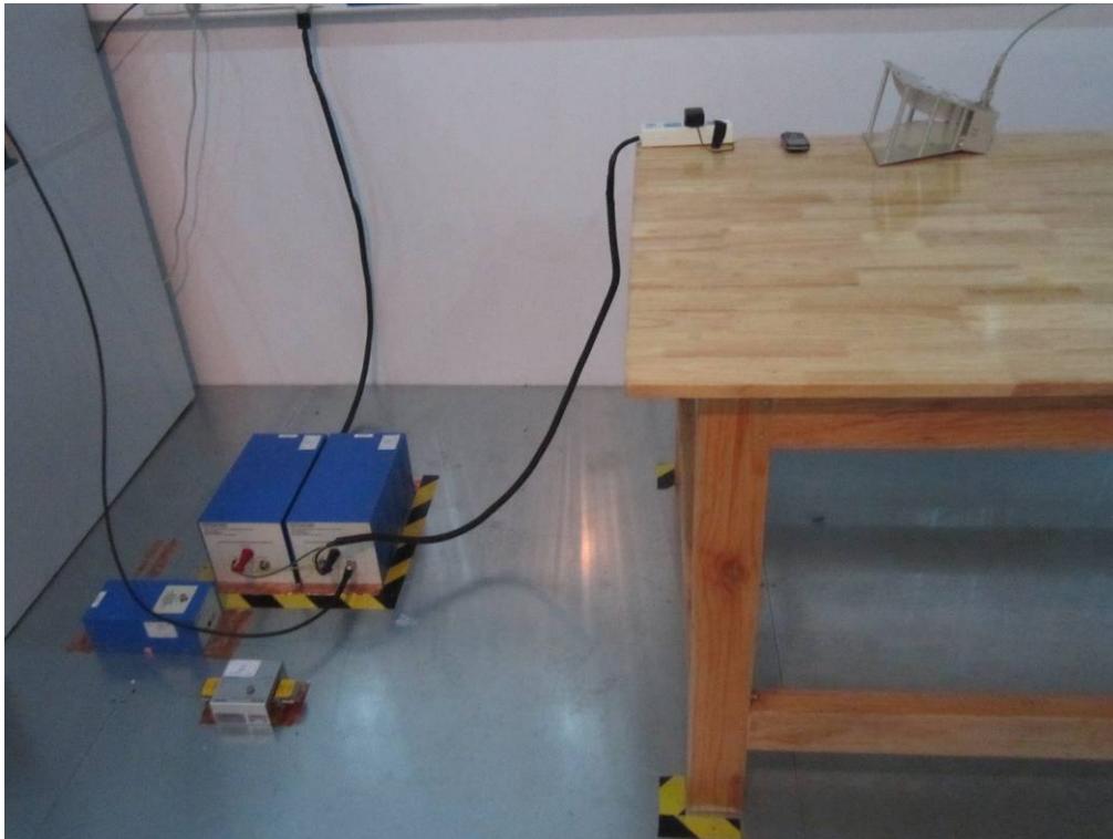
Conducted Emissions Test Setup Front View
