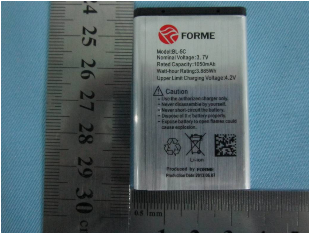
Battery - Top View
