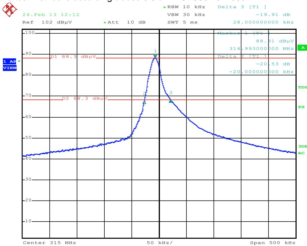
The plot shows the fundamental emission when modulated. From the plot, the bandwidth is observed to be 48.0kHz at 20 dB where the bandwidth limit is  $314.993 \times 0.0025 = 787.48$ MHz.
