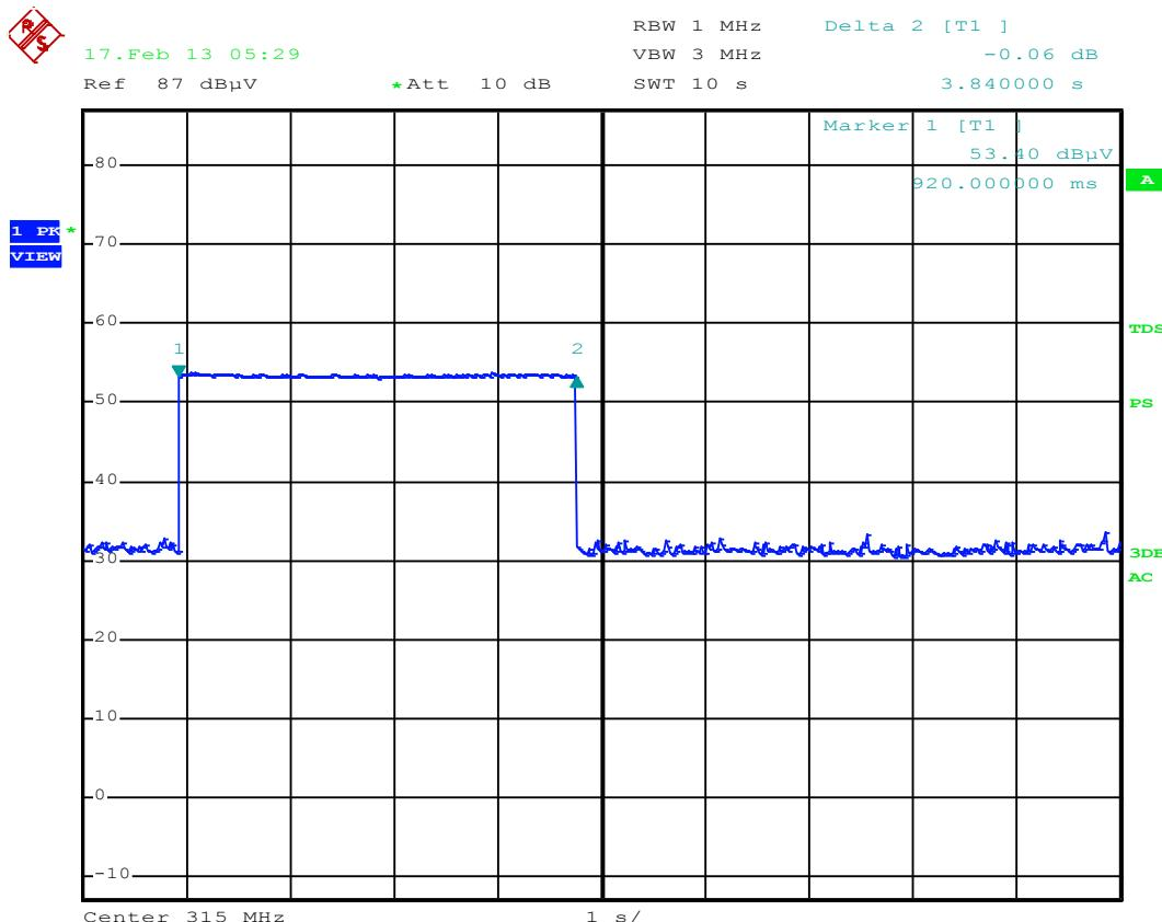
The plot shows the fundamental emission when modulated.
