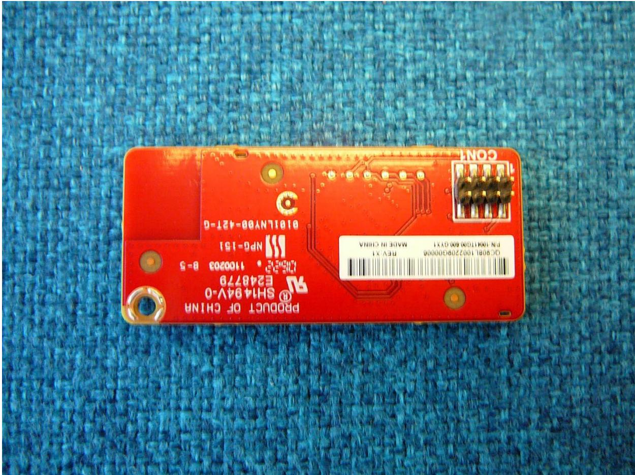
The Qolsys QS-ZW8 Module operates at 908.4 / 916 MHz for US and Canada. It may operate at 919.8 / 921.4 MHz for Australia / New Zealand with an output power up to +4dBm. Data and protocol specifications are beyond the scope of this document. Please contact Qolsys for the technical specifications.
