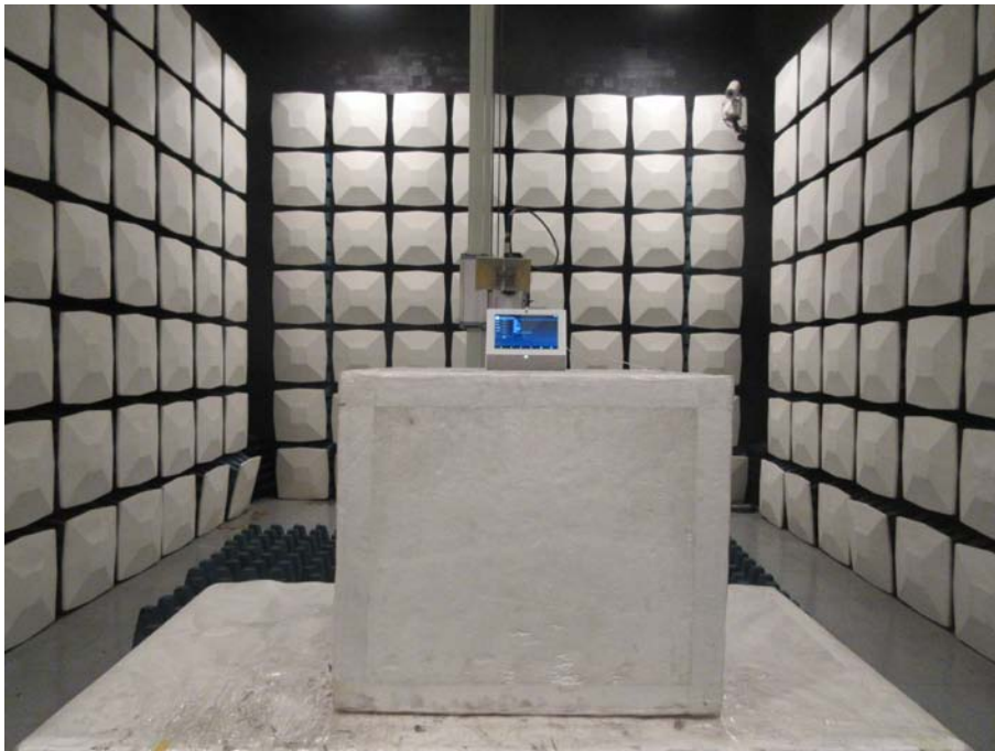
Radiated Emission View (Above 1GHz)
