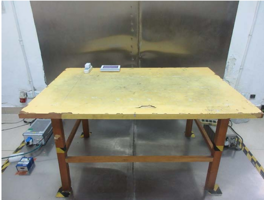
Conducted Emissions Test Setup Front View
