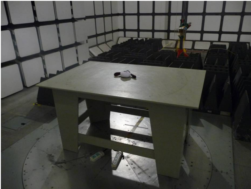
Radiated Emissions View (Above 1 GHz)
