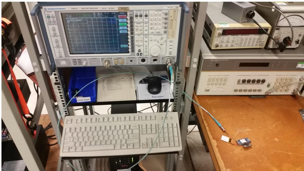
**Radiated Tests Final Setup: In Band Field Strength/Restricted Band Emissions**
