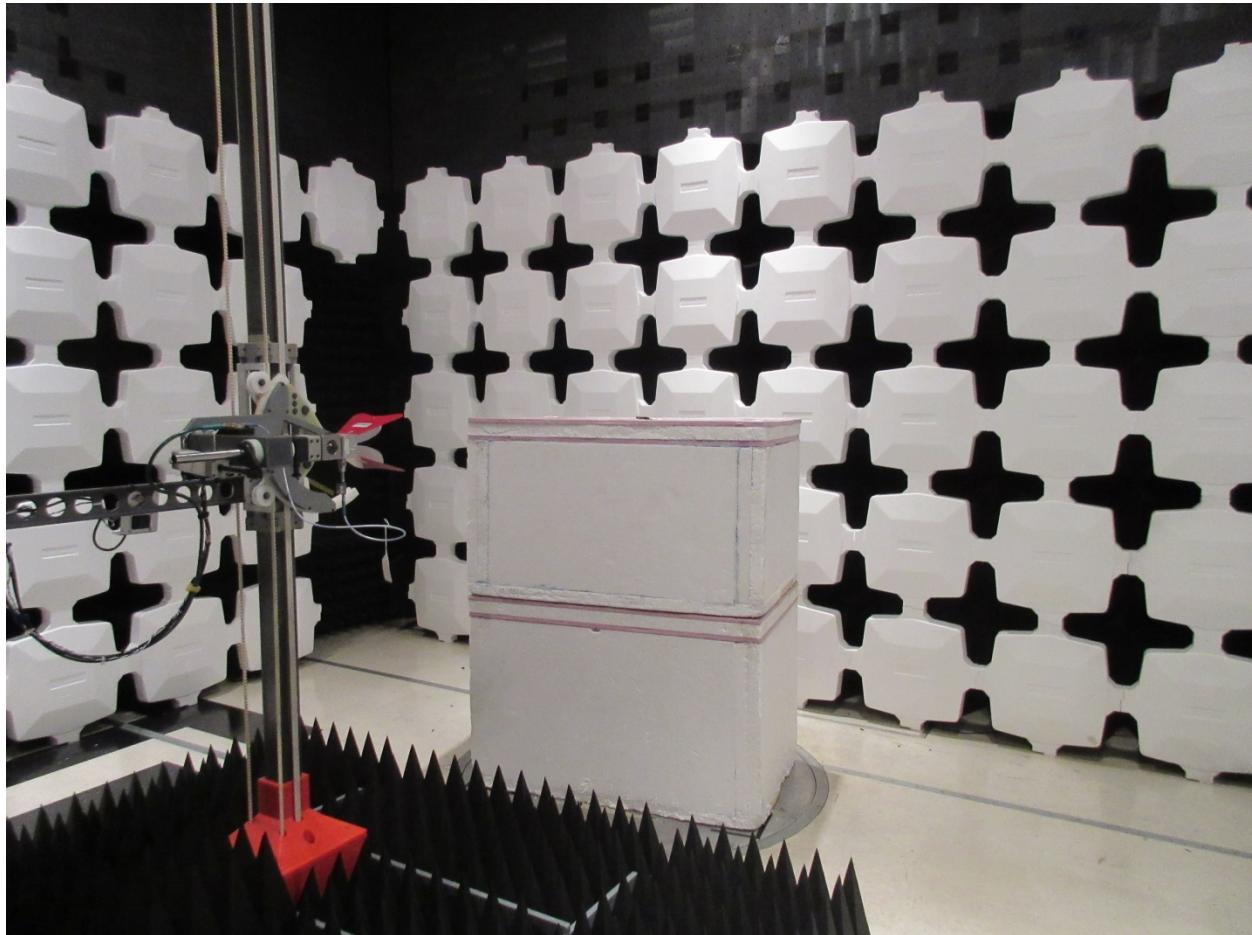
**Radiated Test Below 1 GHz: Restricted Band Emissions**
