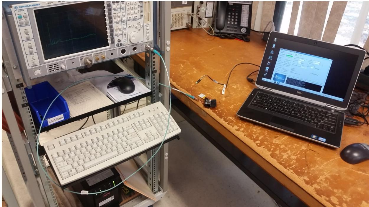
**Conducted Test: Power Output of Fundamental**
