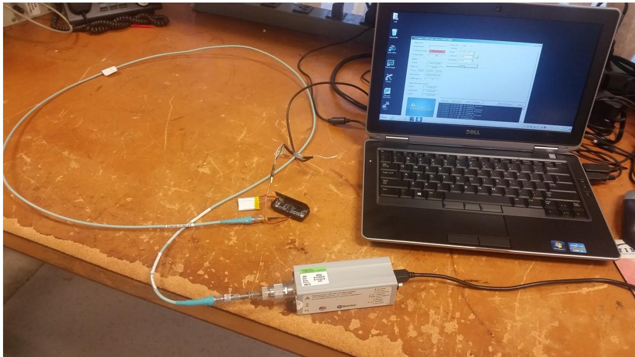
**Radiated Tests Final Setup: In Band Field Strength/Restricted Band Emissions**
