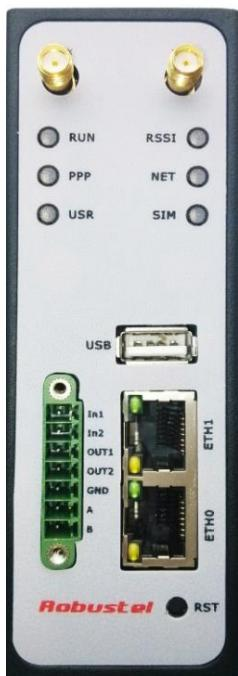
Each Ethernet port has two LED indicators (please check the following picture). The yellow one is **Speed indicator** and the green one is **Link indicator**. There are three status of each indicator. Please refer to the form below.
