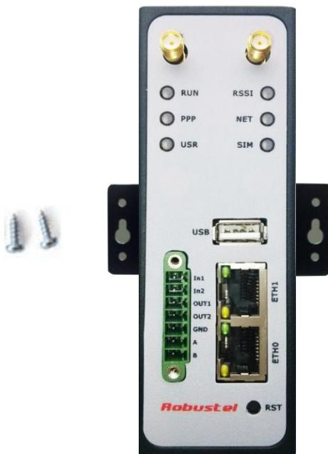
Or mount the router on a DIN rail with 3 M3 screws.
