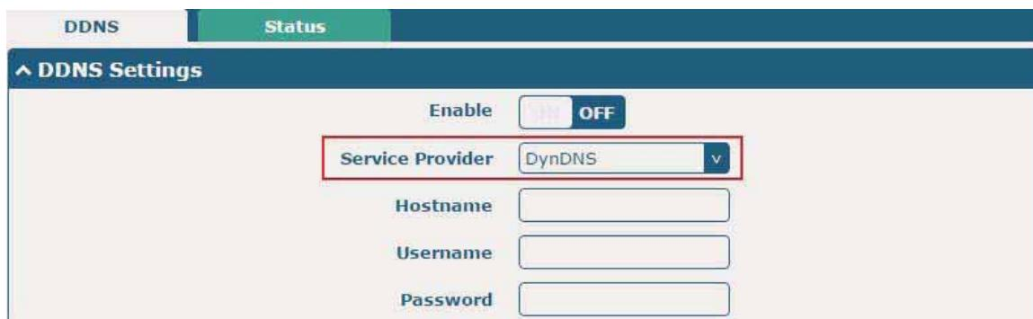
The screenshot shows the 'DDNS' tab selected in the top navigation bar. Below it, the 'Status' tab is visible. The main section is titled 'DDNS Settings' with a sub-section '▲ DDNS Settings'. It contains the following fields:
