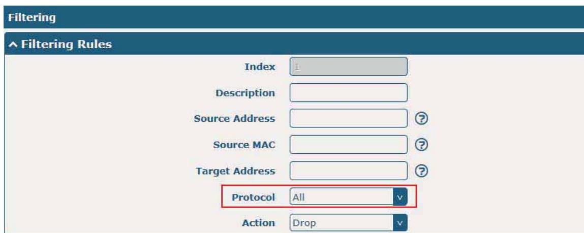
The screenshot shows the 'Filtering Rules' configuration interface. The 'Protocol' dropdown menu is set to 'All' and is highlighted with a red border. Other fields include 'Index' (1), 'Description', 'Source Address', 'Source MAC', 'Target Address', and 'Action' (Drop).
