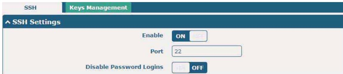
The screenshot shows a navigation bar with 'SSH' and 'Keys Management' tabs. The 'SSH' tab is selected, displaying the 'SSH Settings' section. It includes fields for 'Enable' (set to 'ON'), 'Port' (set to 22), and 'Disable Password Logins' (set to 'OFF').
