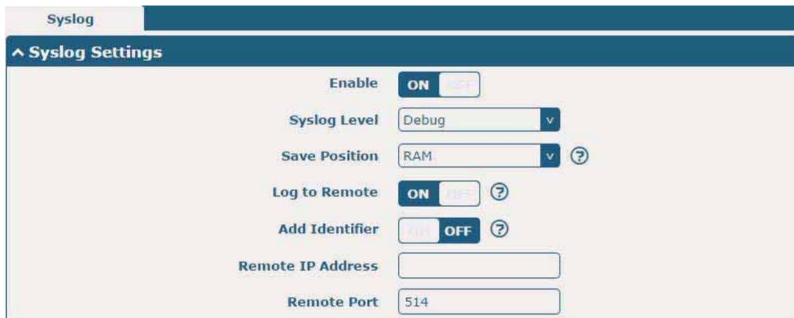
The screenshot shows the 'Syslog Settings' configuration window. The 'Log to Remote' option is set to 'ON' (blue). Other settings include 'Enable' (ON), 'Syslog Level' (Debug), 'Save Position' (RAM), 'Add Identifier' (OFF), 'Remote IP Address' (empty), and 'Remote Port' (514).
