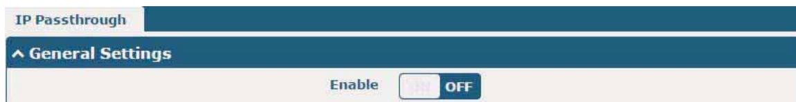
If gateway enables the IP Pass-through, the terminal device (such as PC) will enable the DHCP Client mode and connect to LAN port of the gateway; and after the gateway dial up successfully, the PC will automatically obtain the IP address and DNS server address which assigned by ISP.
