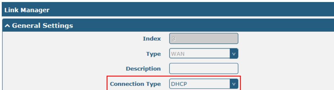
This screenshot shows the 'General Settings' section of the Link Manager for a WAN connection. The 'Connection Type' field is set to 'DHCP' and is highlighted with a red box.
