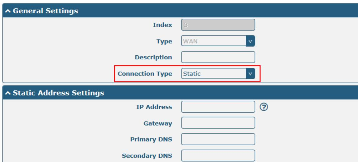
This screenshot shows the 'General Settings' section for a WAN connection with 'Connection Type' set to 'Static', and the 'Static Address Settings' section below it.
