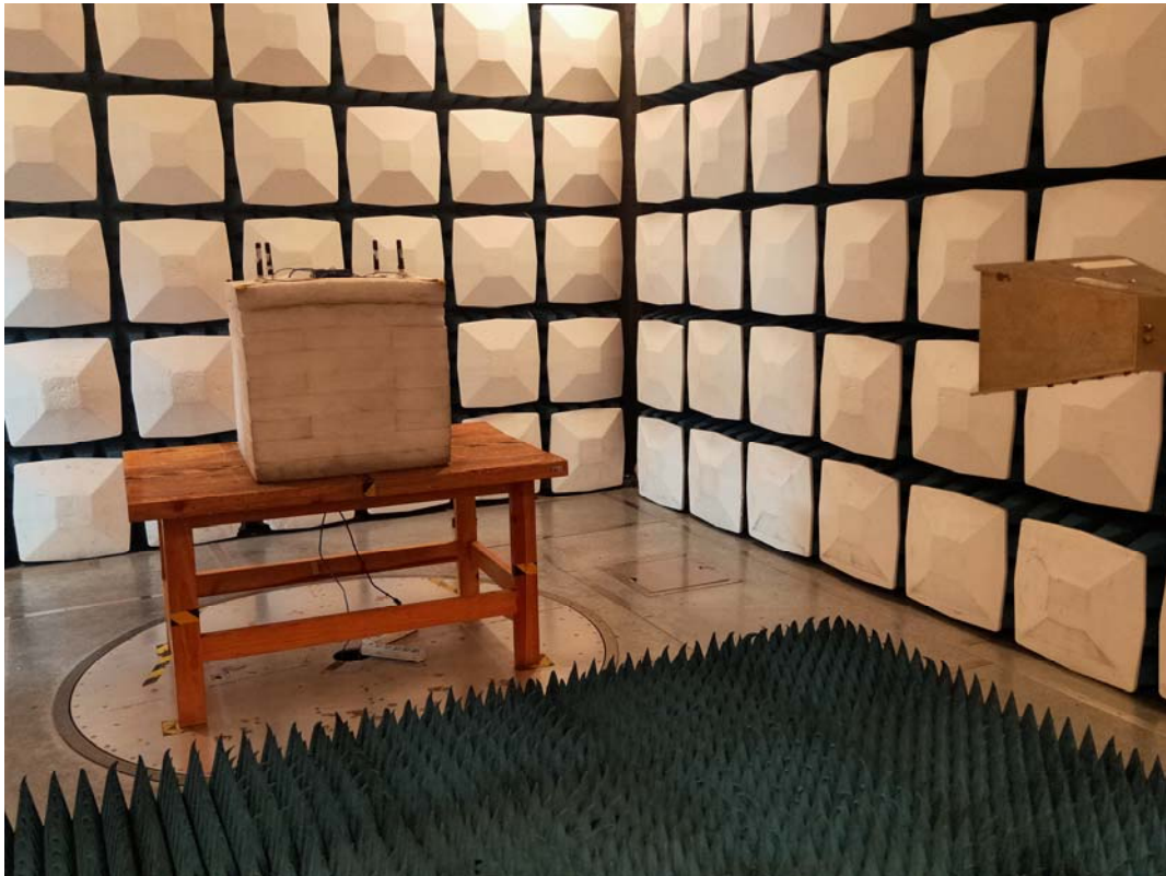
Radiated Emission Above 1GHz View
