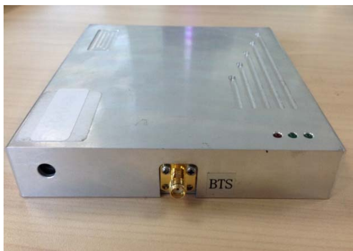
(picture 5) : BTS port: connect to outdoor Antenna
