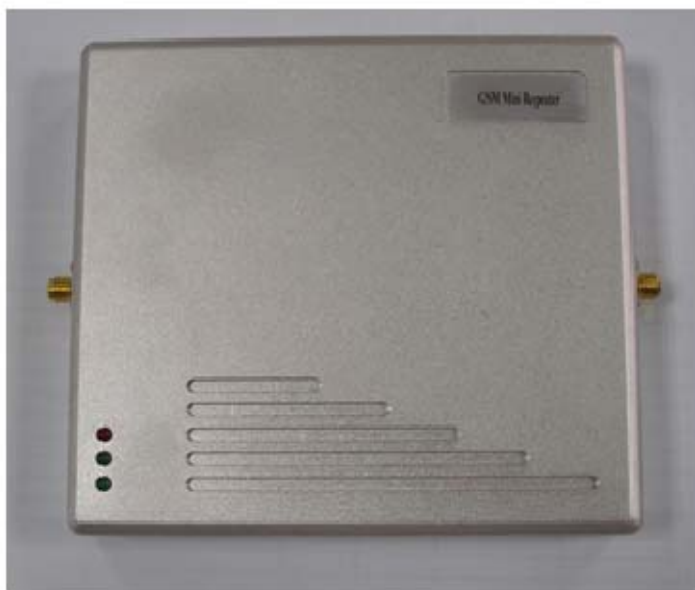
(picture 5) : BTS port: connect to outdoor Antenna
